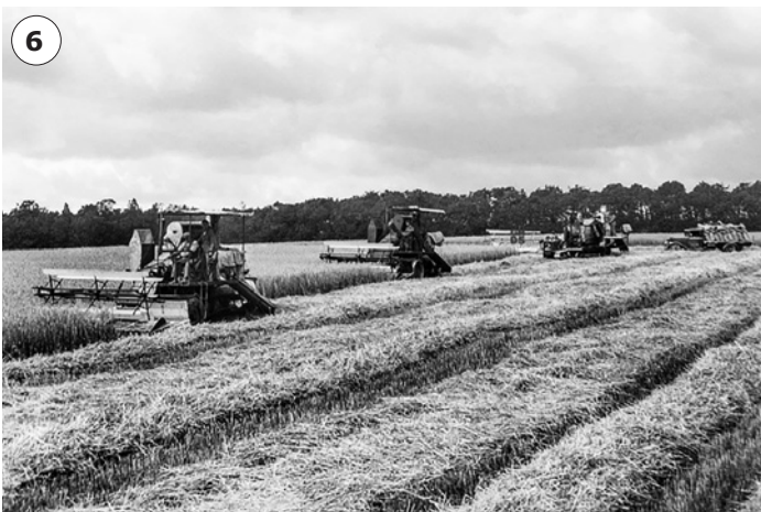
Pic 6: The next step up in tractor design was the specialised combine harvester and, as the three in this picture show, it was a major step. These early combine harvesters left the straw for the baler but took corn itself, which was then loaded into sacks on the back of a lorry. This is basically where we are today, except that nowadays the combines are even bigger, better, more efficient and – best of all – comfortable for the drivers.
