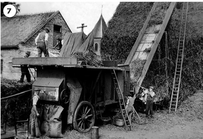
Pic 7: Here we see workers at Merton Grange using an elevator to lift the straw to make stacks in 1940. Over the course of the 20th century, haystacks almost disappeared as most of the straw was burnt in the fields after being cut by the combine harvesters. It was an art in itself to burn a field of straw without burning trees, hedges and sometimes machinery. One man was always in charge of the burning, and would set alight at one corner and burn down and across at the same time, so that the fire would burn itself out.
