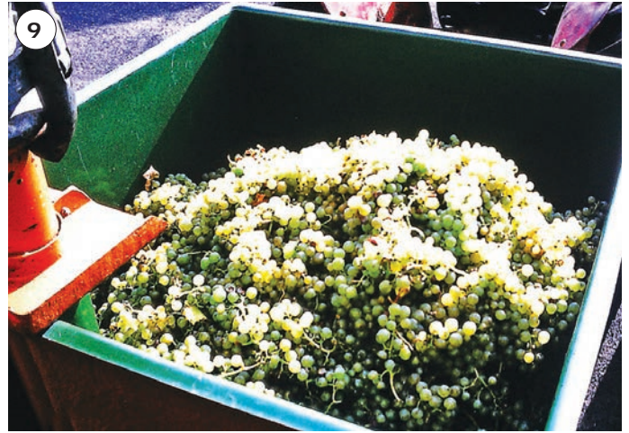
Pic 9: As the grapes were picked they were taken to the winery and put in the grape harvester which had a large mill screw in the bottom which would break the skins so the juice could run freely and then pushed down a large pipe into the cellars and into the press at half a ton per load.
